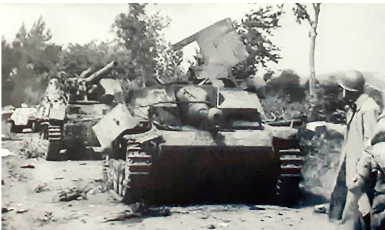
Fig (51) The head of the German column lead by this Panzer IV 'Stug' IV, 75mm SP gun. Note the ripped open armoured panels due to an internal explosion. (Position I) USNA
