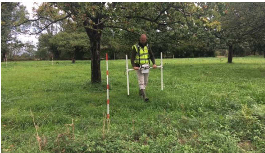
Fig (67) Magnetometer surveys being undertaken at one of the projects sites in Normandy by the project geophysicist using a Bartington Dual Sensor Grad 601-2 fluxgate gradiometer. (BAG)
