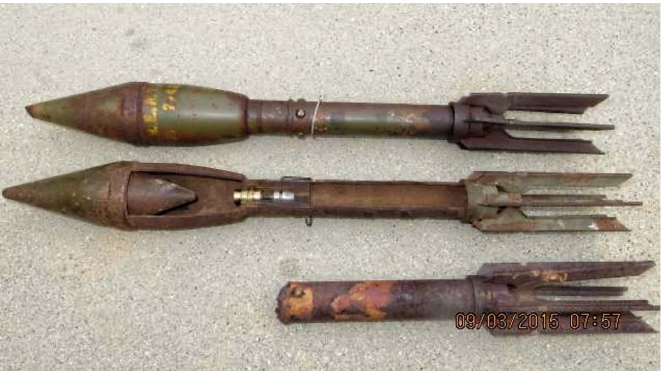
Fig (128) WW2 American 60mm M6A3 Bazoooka rocket examples possibly representing the Rocket found at La Chapelle. (USNA)
